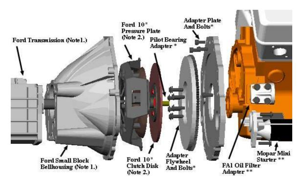
NOTE 1. USE THE FORD SMALL BLOCK BELLHOUSING, THROWOUT BEARING AND LINKAGE (FORK) THAT WERE STOCK TO YOUR TRANSMISSON
