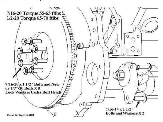
BOLT THE FLYWHEEL TO THE CRANKSHAFT USING THE SUPPLIED 7/16"-20 X 1 1/2" BOLTS AND NUTS (OR ½"-20 BOLTS). REMEMBER WHEN BOLTING THE FLYWHEEL TO THE CRANKSHAFT AND WHEN BOLTING YOUR PRESSURE PLATE TO THE FLYWHEEL PROCEED IN A CRISS-CROSS PATTERN A MAXIMUM OF 1/2 TURN AT A TIME.
