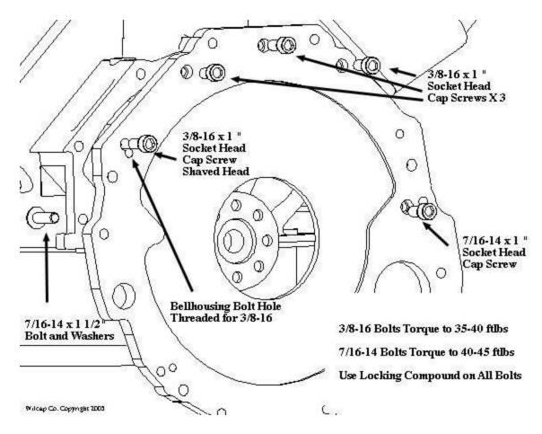
USING THE SUPPLIED 3/8-16 SOCKET HEAD CAP SCREWS & 2 7/16-14 BOLTS, BOLT THE ADAPTER PLATE TO THE BLOCK. IF NECESSARY USE A RUBBER MALLET TO FIT THE PLATE UP TO THE BLOCK FLUSH. DO NOT USE THE CAP SCREWS TO FORCE THE PLATE ONTO THE BLOCK. CHECK FOR FIT. THE PLATE SHOULD FIT FLAT TO THE ENGINE BLOCK WITH NO ROCKING OR GAP.
